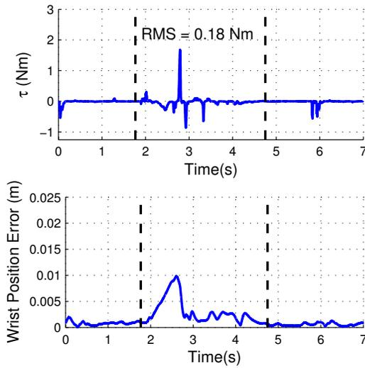
Fig. 7. Wrist torque  $\tau_e$  and position error  $|\vec{x}_{error}|$  during typical low impedance peg insertion shows smaller insertion torques.
