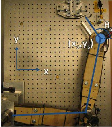
Fig. 3. Planar 3-DOF slave device with wrist mounted force sensor.
