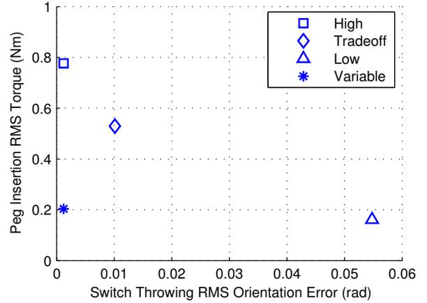
Fig. 11. Relative performance of the impedance configurations quantified via RMS  $\tau_e$  during peg insertion and RMS  $\theta_{error}$  during switch throwing. Variable  $k_{p,\theta}$  achieves the best performance possible in both tasks.
