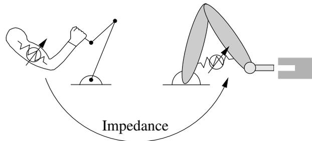
Fig. 1. Variable impedance manipulation involves continual adjustment of the robot's impedance throughout task execution
