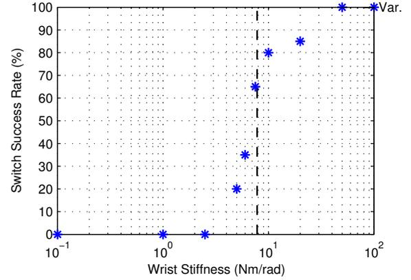
Fig. 9. Switching success percentage increases with wrist stiffness  $k_{p,\theta}$ . The predicted value of stiffness required is marked as a vertical line. Variable impedance had 100% success, as marked on the y-axis.
