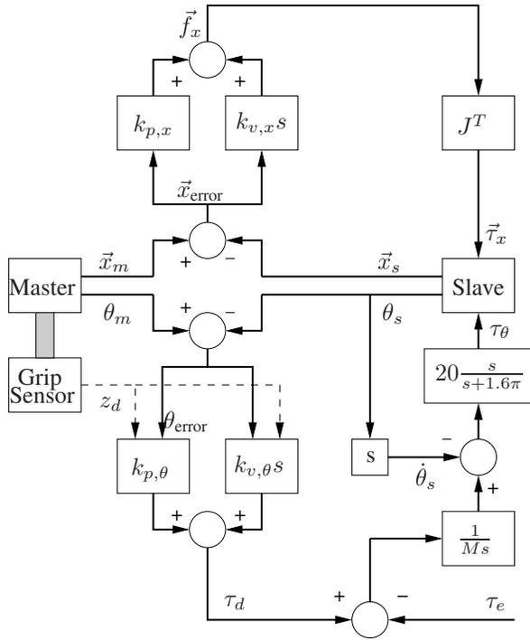
Fig. 2. Telerobotic architecture with separate control for position and orientation. The master is unactuated so that the low frequency slave orientation impedance is determined only by  $k_{p,\theta}$  and  $k_{v,\theta}$ .
