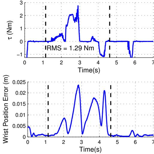
Fig. 6. Wrist torque  $\tau_e$  and position error  $|\vec{x}_{error}|$  during typical high impedance peg insertion shows stick-slip and jamming in the position trace.
