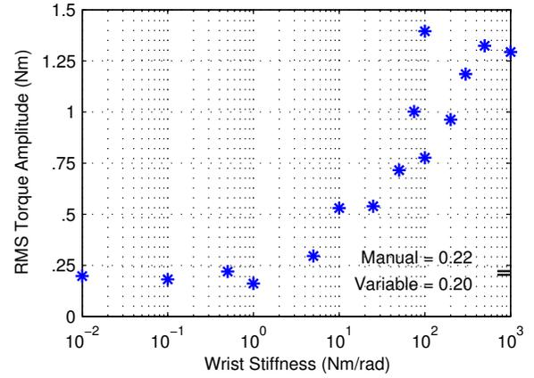
Fig. 5. Wrist stiffness  $k_{p,\theta}$  versus RMS wrist torque  $\tau_e$  during peg insertion shows that insertion torque increases with stiffness. RMS  $\tau_e$  values for manual and variable impedance peg insertion are labeled and marked on the y-axis.
