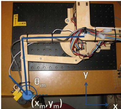
Fig. 4. Planar 3-DOF master device with grip force sensing.
