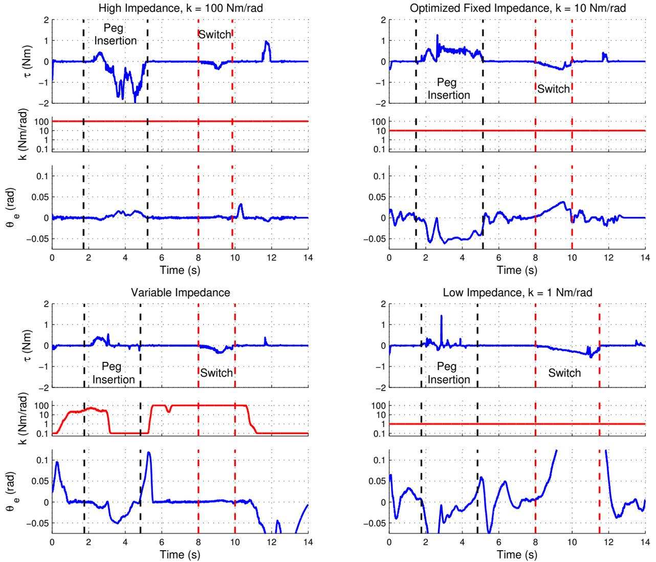
Fig. 10. Wrist torque  $\tau_e$ , stiffness  $k_{p,\theta}$  and orientation error  $\theta_{error}$  during combined task execution for high, medium, low, and variable impedance. Vertical lines highlight insertion and switching tasks. Only variable impedance achieves the lowest insertion  $\tau_e$  and smallest switching  $\theta_{error}$ .
