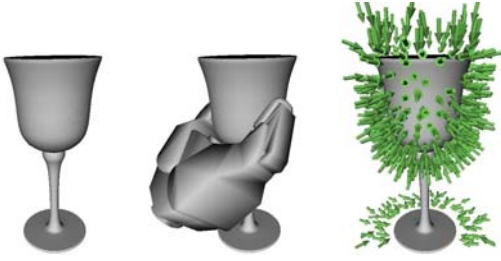
Fig. 4: Database-driven grasp planning: the object model, an example grasp and the complete set of computed grasps.
