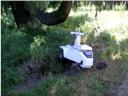
Fig. 1. Our robot in typical terrain. Robot is part of a DARPA project, Learning Applied to Ground Robots(LAGR). Two stereo systems are on the upper crossbar.
