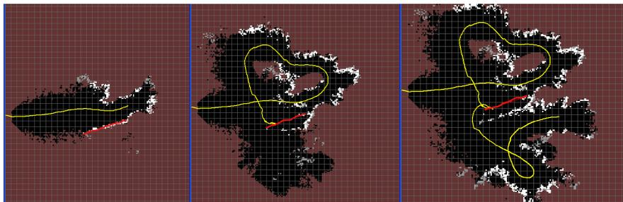
**Fig. 6.** Three stages during a run using GPS filtered pose. Obstacle points are shown in white, freespace in black, and the yellow line is the robot's path. The linear feature is marked by hand in red in all three maps, in its initial pose.
