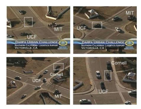
Figure 22. (Clockwise from upper left) Little Ben performs a right turn while passing a robot vehicle stopped in the wrong lane.
