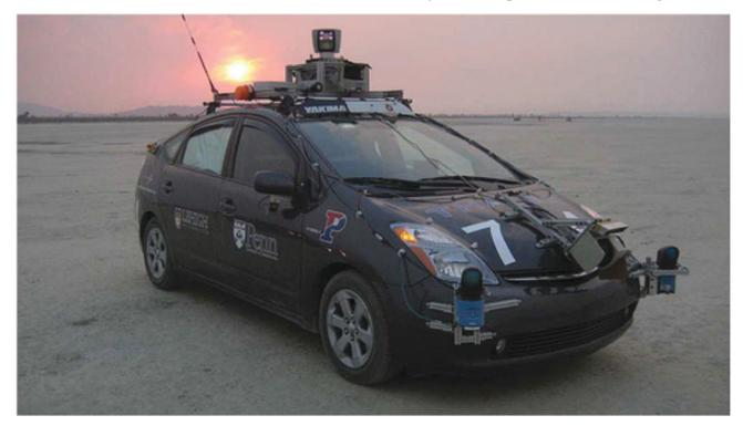
**Figure 1.** Little Ben is a Toyota Prius hybrid vehicle modified for drive-by-wire operation with an onboard array of sensors and computers.
