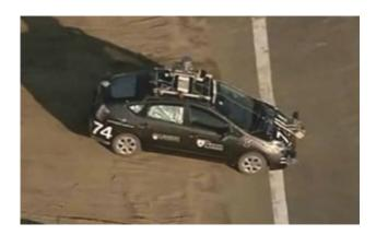
Figure 21. Little Ben temporarily stalled on the transition from the Outback to Phantom Road East. The steep pitch of the transition resulted in the road surface being falsely classified as an obstacle.
