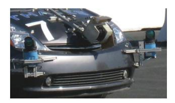
**Figure 6.** Sensors mounted on the hood of Little Ben.
