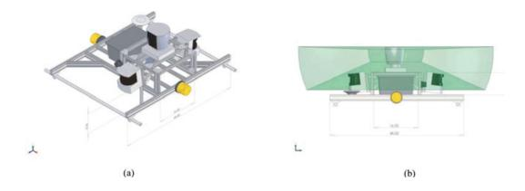
**Figure 5.** Roof sensor rack designed to provide optimal viewing angles.
