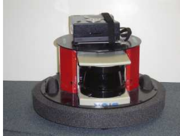
Figure 1. The Botrics Obot mobile robot, equipped with a SICK scanning laser range-finder, which has a 180^\circ sensor field.
