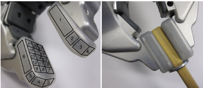
Fig. 7: Arrangement of the pressure sensors on the finger pads (left) and closeup of the placement of the chopsticks in the gripper (right).
