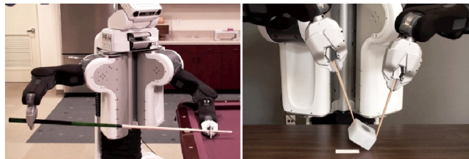
Fig. 1: The PR2 robot learning a pool stroke and manipulating a box using chopsticks.
