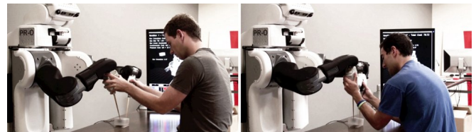
Fig. 8: An informal user study was conducted: 10 subjects were asked to flip the box by guiding the robot's gripper and only an average of 3 out of 20 attempts were successful.
