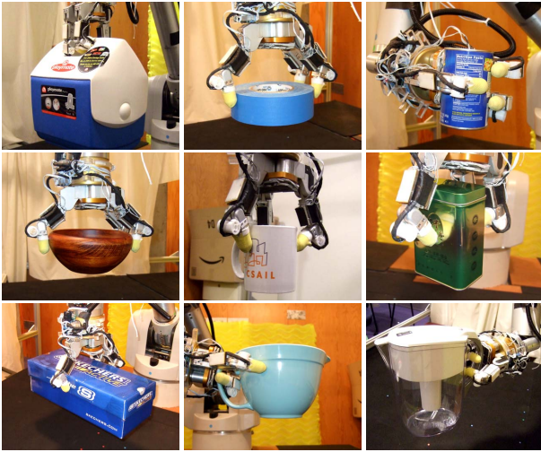
Fig. 1. Goal grasps for all objects except power drill.
