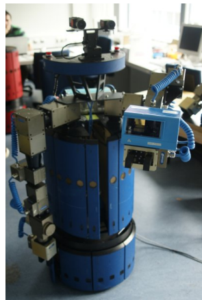
Fig. 1. Autonomous robot used for the experiments in this article. A SICK laser scanner is mounted on the left robot arm, which allows the robot to acquire 3D scans of the environment by sweeping its arm.
