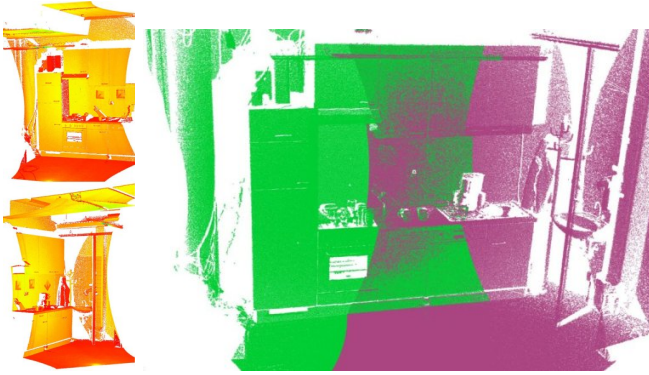
Fig. 5. Two separate scans of the kitchen (left), and the resulted model after registration (right).
