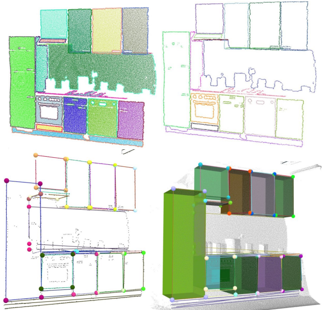
Fig. 9. Boundary points of each segmented planar region (top); 4 best fitted lines to each region boundary (bottom left); Cuboids created by projecting the 2D quad on the wall (bottom right).
