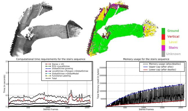
Fig. 2. Top: a snapshot of the point cloud data and semantic model for the stairs data set; bottom: computational time and memory usage requirements per useful stereo frame.
