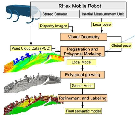
Fig. 1. The overall system architecture. obtained on the stairs dataset, together with its computational properties.
