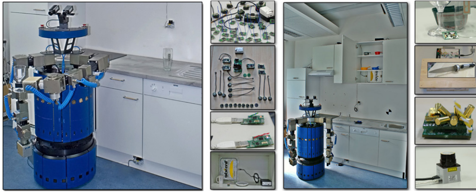
Fig. 2. A snapshot of the AwareKitchen hardware architecture.
