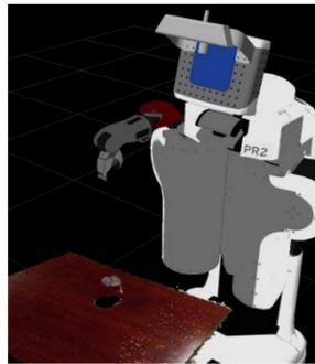
Robot uses visual object recognition to get an initial pose and shape distribution for the object.
