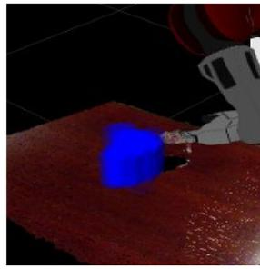
Contact is made, and now the pose and shape of the object are quite certain. Robot plans a new grasp once more to do the final pickup.
