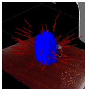
No contact is made (object is shorter than expected), so grasp is aborted and a new grasp is planned based on updated object distribution.
