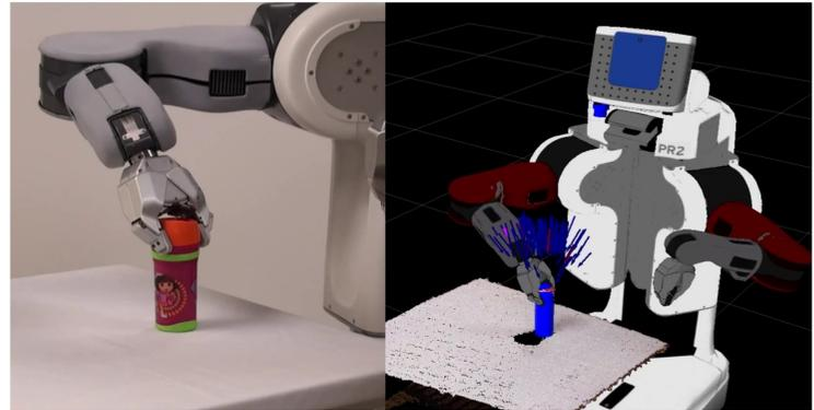
Object on table (as seen by Kinect point cloud) has uncertain shape/identity and pose.
