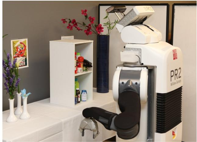
Figure 6: The PR2 robot preparing to execute a grasping task in our experiments. This difficult scene includes large obstacles and a highly-cluttered arrangement of objects in the shelf.
