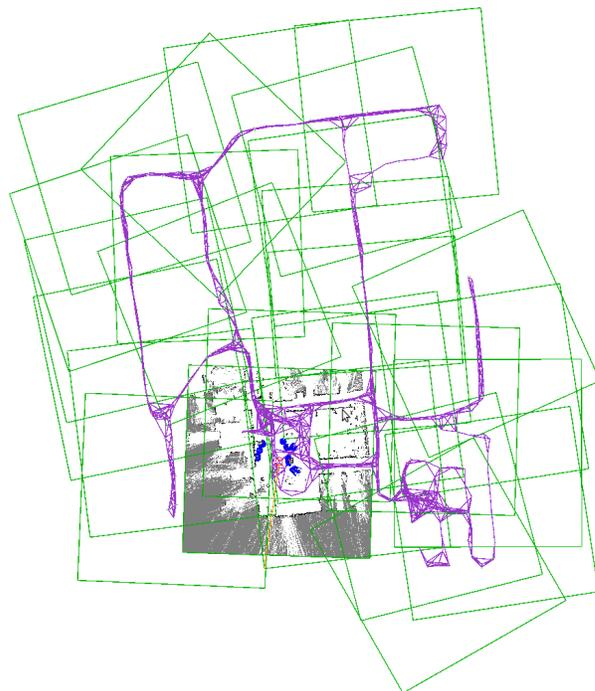
Fig. 5. The navigation graph generated for the simulation environment in which experiments were performed. The green boxes represent the local grids stored in the graph. The grid with obstacle information displayed is the active grid for the metric navigation system.
