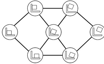
**Fig. 1.2.** A complete contact state graph shows all possible CFs (nodes) and transitions between neighboring CFs (arcs). While this figure shows a simplified example that only contains 7 CFs, a real contact state graph of two 3-dimensional polyhedral objects contains hundreds of CFs.
