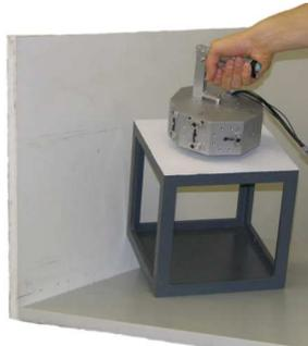
**Fig. 1.3.** The demonstration tool is manipulated in contact with three perpendicular faces. The Krypton K600 optical system uses three cameras and triangulation algorithms to measure the spatial position of each of the LED markers on the demonstration tool.
