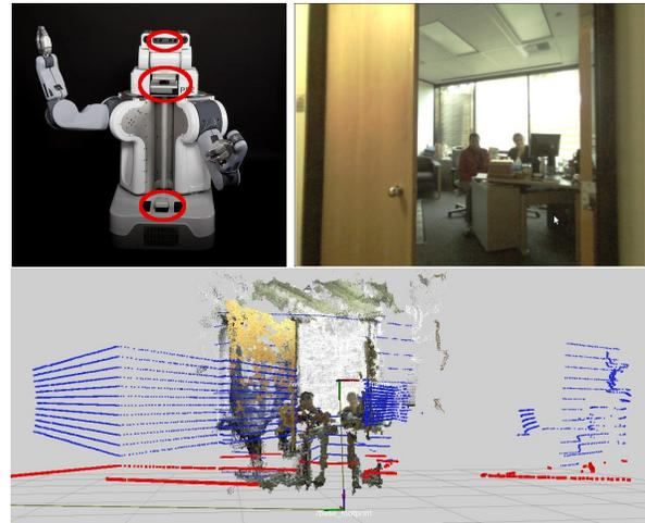
**Figure 1: The PR2 robot with sensors used for data collection circled (top left); Image from the MPMP Dataset (top right); Corresponding laser and stereo data snapshot (bottom). (Best viewed in color.)**
