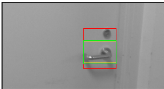
Fig. 5. Vision door handle detection. The green box is the final detection vote over seven frames, with intermediate detections represented by yellow boxes. The red box is a false detection filtered out by scale considerations.
